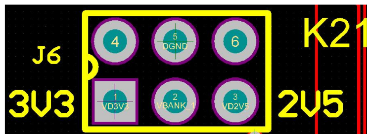
Figure 4a – Pin allocation of J6 (J12 is identical)
